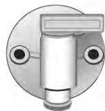
Exterior Fresh Water Drain
