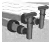
Low Point Drains
