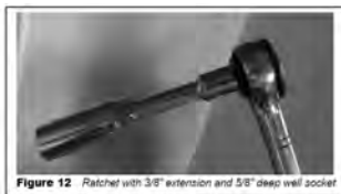
Figure 12 Ratchet with 3/8" extension and 5/8" deep well socket
