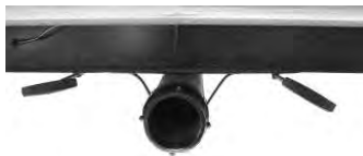
Black/Grey Tank Drain and Valves
